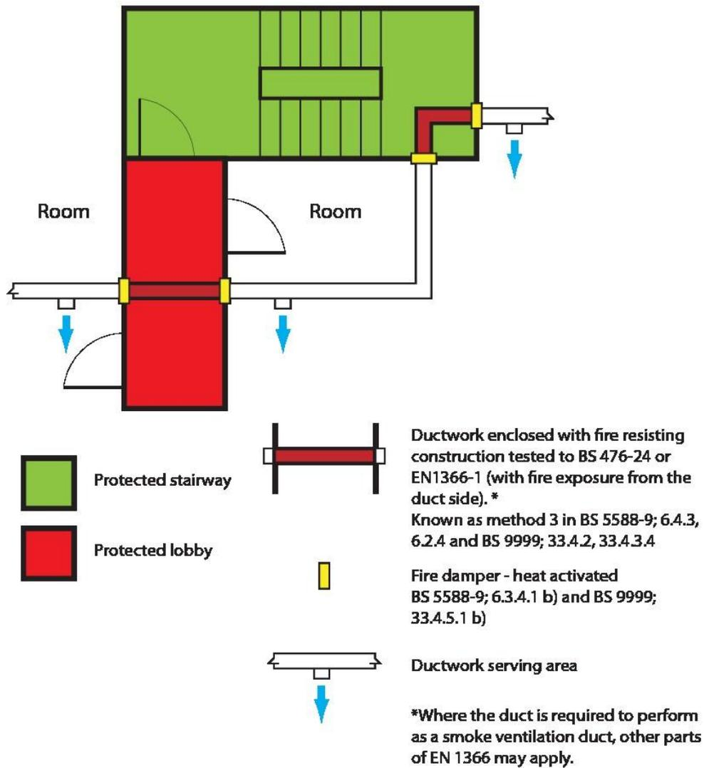
**Figure 2 - Protected ductwork solution - Method 3 - Ductwork passing through protected routes without serving the route (Method 3 in BS 5588-9; 6.4.3 and BS 9999; 33.4.3)**
