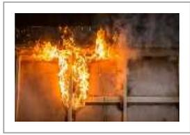
The fires involved rapid vertical fire spread via combustible cladding finishes and insulation, exacerbated by vertical cavities and a plentiful supply of combustion air. As facade fires are all too common, it is increasingly important that fire risk is taken into account at the design stage. Exova Warringtonfire recommends four suitable options to provide an acceptable cladding system:
