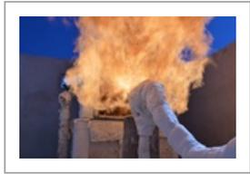
The **Applus+ Fire Laboratory** has put into service new facilities for undertaking open-field tests. Applus+ is now able to safely conduct Jet Fire Tests under standard ISO 22899-1 that could not be carried out in a conventional fire laboratory.
