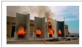
Recent fires in high-and mid-rise buildings demonstrate the importance of the characteristics of the facade. Factors such as surface quality and cavities, etc can play a decisive role in the event of a fire, with the cladding system and facade facilitating the spread of the fire.
