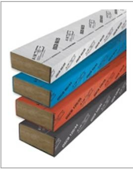
Manufactured from ROCKWOOL stone wool and faced with intumescent material, the AIM OSCB provides an open airspace of 25mm and 44mm. When installed the OSCB allows air flow in the facade cavity, with the intumescent strip expanding to create a robust cavity fire barrier, in the event of a fire.
